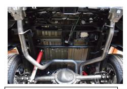
6. Install supplied 2-1/2" band clamp(Item I) onto the inlet side of both the Driver and Passenger side exit pipes(Item G, F) and install them onto the outlets of each over-axle pipe. Tighten both clamps with allowance for adjustment.
