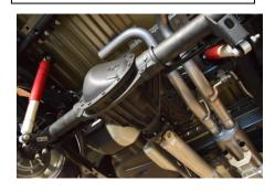
5. Install supplied 2-1/2" band clamp(Item I) onto the inlet side of the driver side over-axle pipe A(Item D) and install onto outlet of muffler. Install hanger into factory rubber grommet hanger. Next install another 2-1/2" band clamp(Item I) onto the inlet side of driver side over-axle pipe B(Item E) and install onto outlet of Item D. Tighten both clamps with allowance for adjustment.
